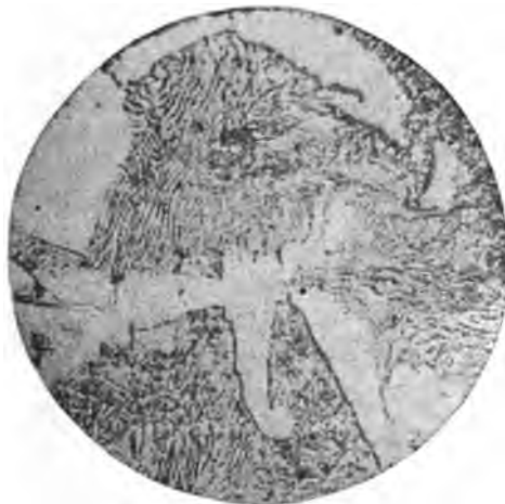
FIG. 46. — White Cast Iron. Magnified 500 Diameters. (Wust.)
